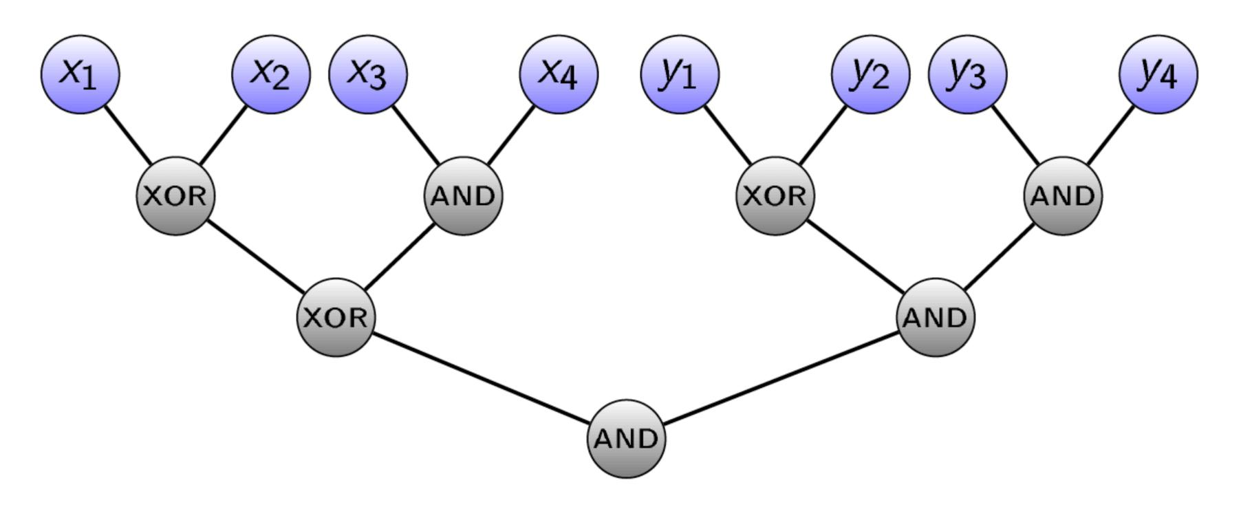
Idea: « encrypting » the gates such that they can only be evaluated given appropriate keys, and while hiding their exact behavior.
